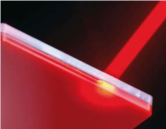
Plastics Welding with Mid-IR Wavelength
