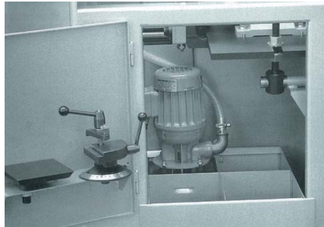
The high capacity coolant pump is mounted directly on the pull-out coolant tank
