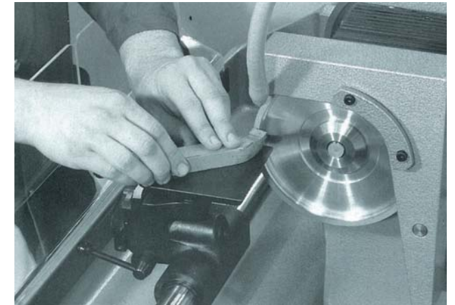
Off-hand radius grinding. Tool on grinding table, item 4.01.73.00
