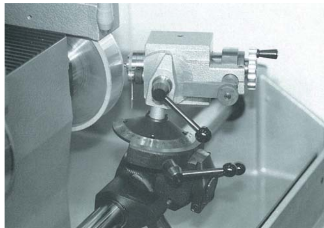
Cutter grinding attachment, item 401.82.50.0, for cylindrical and conical grinding. Multi-facet grinding with dividing disc, face and radial relief grinding, with W20 collets
