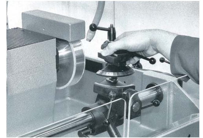
Rapid changeover of accessories. Tool holder 15, item 3.00.49.40, placed in basic adapter
